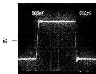
MAX406 LARGE-SIGNAL TRANSIENT RESPONSE (DECOMPENSATED MODE)
