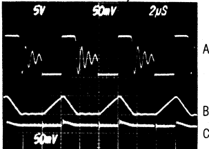
MAX752 SWITCHING WAVEFORMS DISCONTINUOUS CONDUCTION
