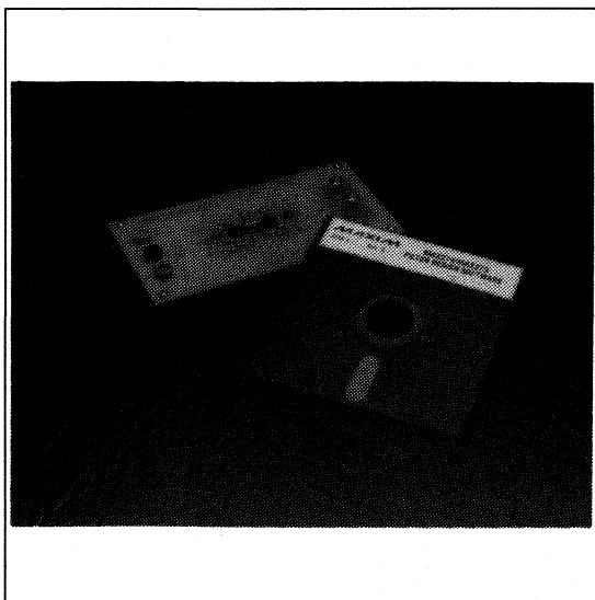
Figure 1. The MAX274 EV kit includes filter design software, PC board with MAX274 IC, and full documentation.
